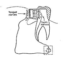
Figure 3 By 1964, Puharich had improved the amplifier so that it could be mounted on the back of the tooth. In this drawing, the amplifier "is greatly exaggerated in size to facilitate description" and would, in fact, be hidden under the tooth cap. The amplifier has a terminal on the left which must be touched with the tongue to complete the circuit. Drawing from US Patent 3 156 787
