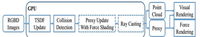
Fig. 3: The haptic rendering pipeline: collision detection method [16] is used; a new proxy update method is used to find proxy; Friction and texture are added to simulate the properties.
