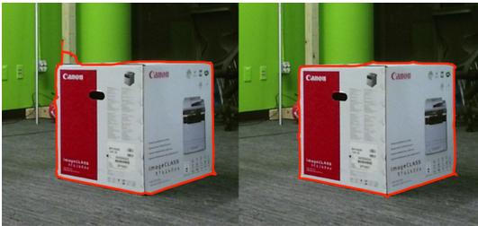
Fig. 7: Interactive region growing 2D segmentation method. Left is only using RGB image, right is using both RGB image and depth image, which keep the better boundary for the object.
