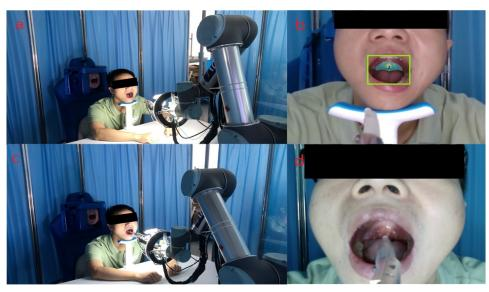
Fig. 9: Sampling process from vision detection to sampling tasks. In our experiments, many volunteers were tested, and the recognition rate, control precision, sampling time, and sampling contact force were recorded.
