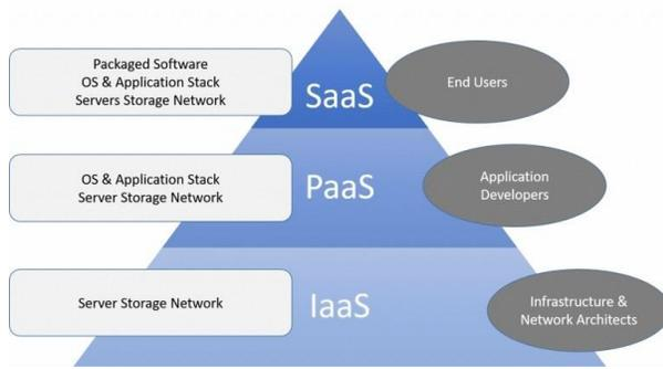
Figure 2. Cloud Computing Operational Service Models
