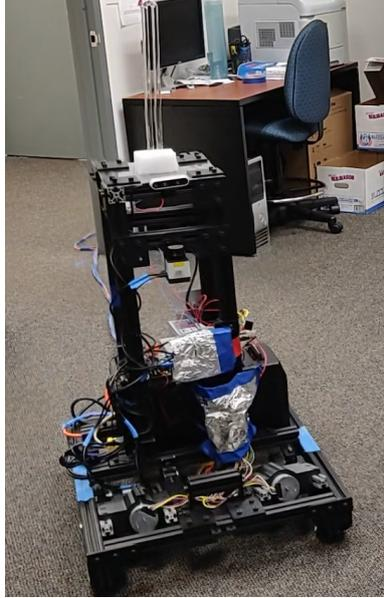
Figure 2: The robot developed for autonomous UVC irradiation driving into a room to be disinfected.
