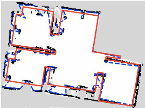
Figure 3: Comparison of Douglas–Peucker (blue) and rectilinear (red) simplifications, overlaid with the grayscale grid obtained the ROS GMapping algorithm.
