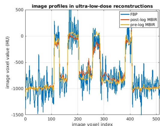
Fig. 3. Image profiles through the center of reconstructed images from the ultra-low-dose data. The FBP image is extremely noisy. The post-log MBIR image contains much less noise but shows strong bias on the order of 100 HU in the central area. The pre-log MBIR image gives remarkable improvement of HU accuracy when compared with post-log MBIR.
